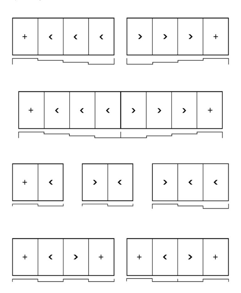
Endless Fixed and Sliding Panel Configurations.
